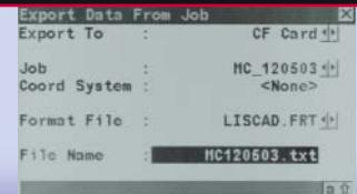
Data can be exported directly from GPS1200 or via Leica Geo Office in various standard formats or in your own user-defined formats for direct input into any type of processing, office, CAD or mapping software.
