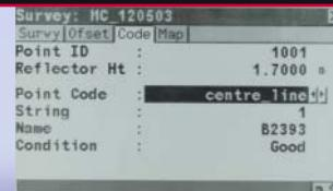
Define points, lines and areas to build up a plan in the display as you survey. You see immediately what you've done. Attach the codes, attributes and information needed for input into your office or mapping software.
