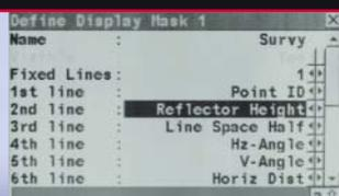
With GPS1200 you can define different display masks so that the system shows exactly what you and your crews want to see when surveying in the field. Set the displays according to the jobs you do and the information required.
